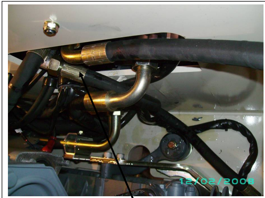
Hydraulic line rerouted under 90° hydraulic elbow.
