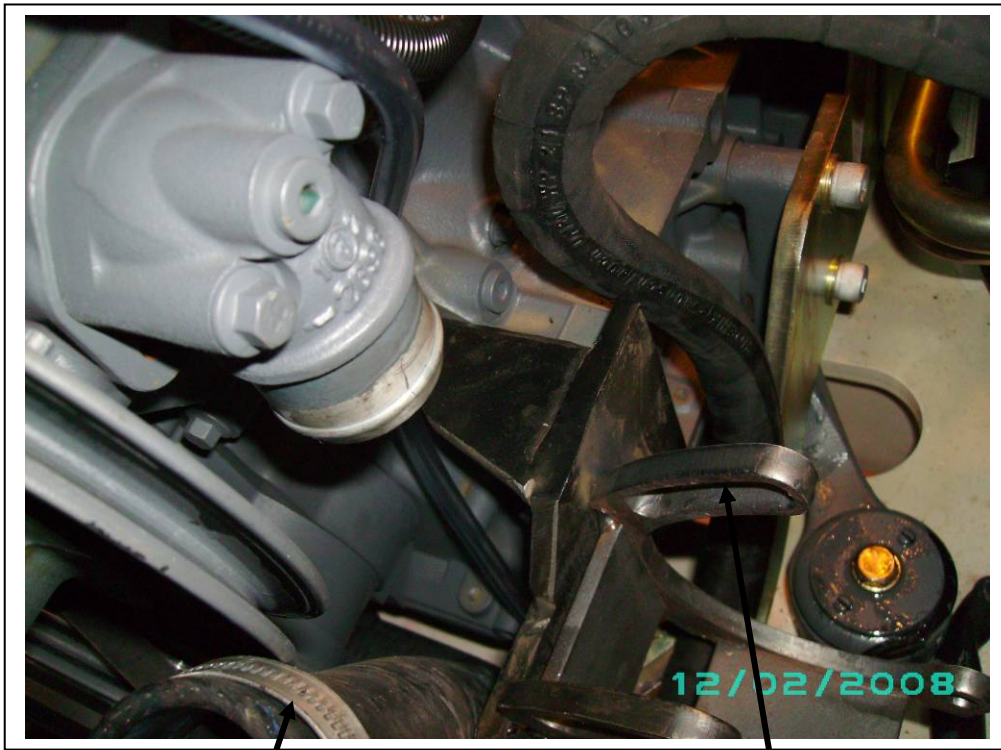
Lower radiator hose removed from engine to allow easy access to the three main mount bolt points.
