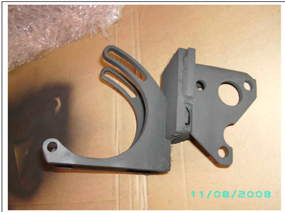
Main mount bracket with three M10 mounting holes showing engine side.
