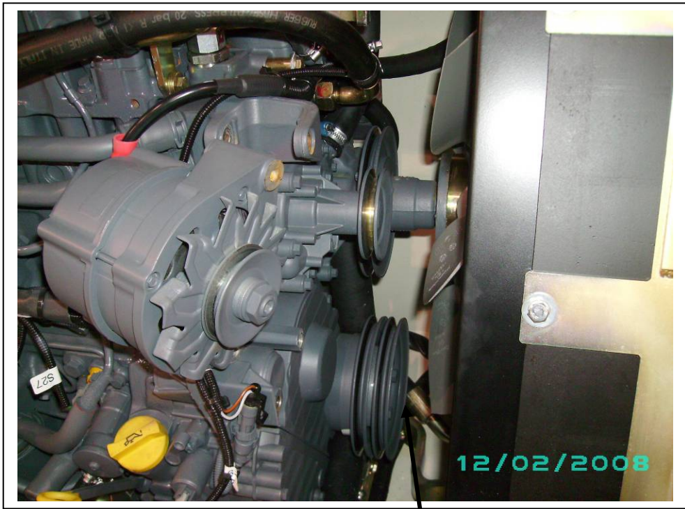
Remove existing four bolts on crank pulley to install an extra crank pulley.
