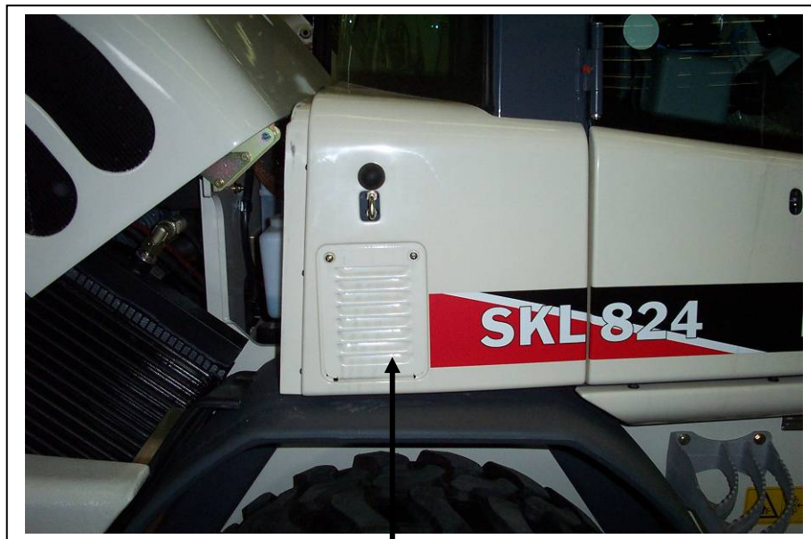
Air intake panel back in place.
